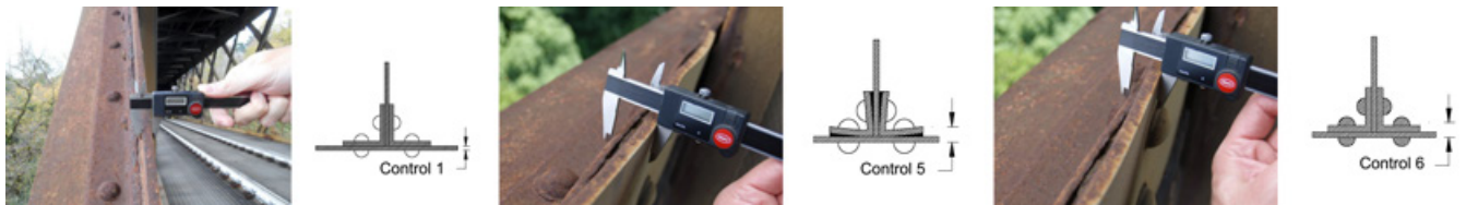
fig.6: Details of the controls of the iron members (© Saisi and Gentile)
